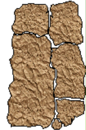
Peds stacked around each other to form soil structure
